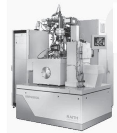
Figure 5.10 Schematic of an electron beam lithography/mask making tool (left). The machine on the right is a Raith product EBP5200 used for both direct writing on wafers and mask writing. Photo courtesy Raith Corp. Reprinted with permission.
